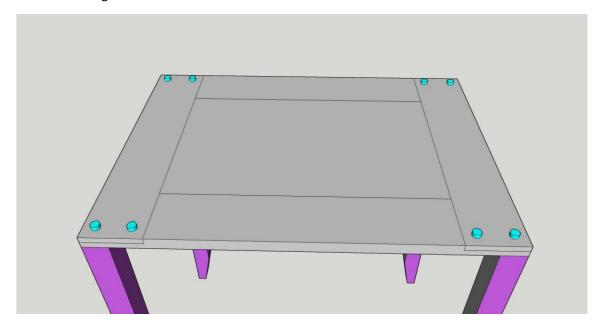
• Using a hand saw, cut off the excess dowel head then sand flush
