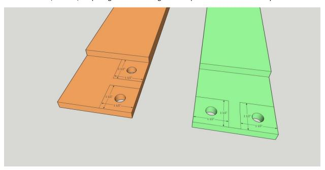
**Pro Tip** – Temporarily assemble (tape or clamp) your half lap joints to make the  $17.50^{\circ}$  x  $24^{\circ}$  frame before drilling the holes for the dowels. If you try to pre-drill before assembly your holes might not line up perfectly.
